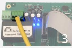
3. Connect cable under O2 Sensor on the V13 print board. The ports are labeled according to the corresponding wire color.
