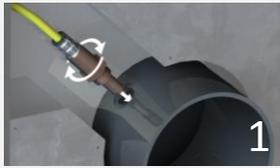
1. Remove stopper from exhaust and screw in the lambda sensor
