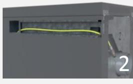
2. Thread the lambda sensor cable through cable track and connect to the print board
