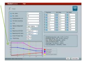
Weather compensation is a method to adjust the flow temperature to the actual needs from the outside or inside temperature. The idea is that the colder it is outside, the warmer the flow for heating the house needs to be, or vice versa, the hotter it is outside, the "cooler" can the flow be. It is not only the outside temperature that determines the need, but the wind's cooling effect (chill factor) also has a great significance
